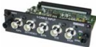
Image 5-6 5 Cable input (Multi purpose) (R9854435).
